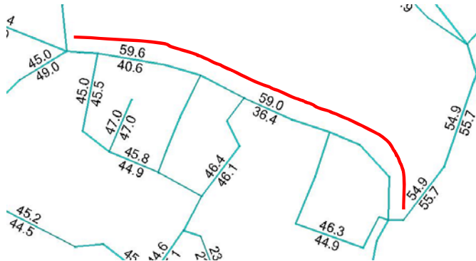
Figure 2: Modelled speed in morning peak hour (Base scenario).
