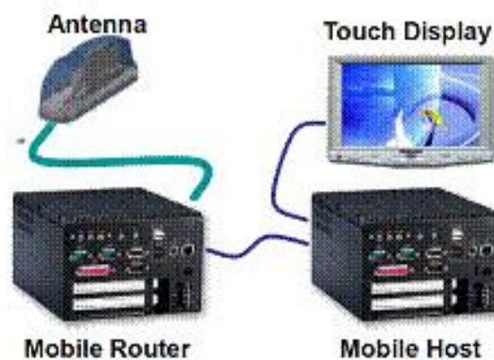
Figure 3 CVIS reference platform components
