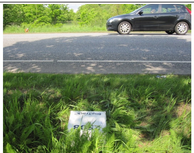
Figure 4 - The Bluetooth sensor located on the ground at West-East Shoulder at Sauervej-Scoresbysundvej (Point B).
